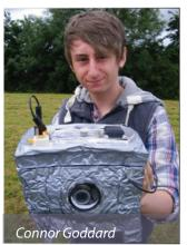
The balloon was equipped with a digital camera which captured images throughout the ascent, electronic sensors to gauge temperature and atmospheric pressure, and a GPS module to relay positional data allowing the team to track the balloon as it climbed.
