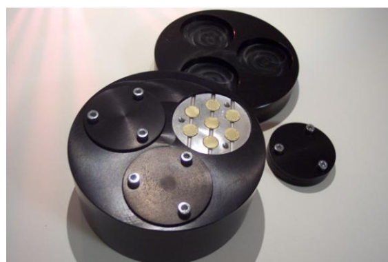
Figure 5: An adapter for a laboratory sieve shaker which holds 3 single grain disc holders.
