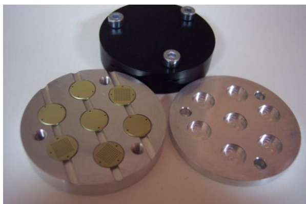
Figure 2: Single grain disc holders to help with the cleaning process and to store the discs.
