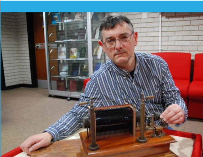
Professor Iwan Morus with an induction coil which were in use from the 1830s. Between around 1890 and 1920 they were used to generate high voltage to create electromagnetic (radio) waves.
